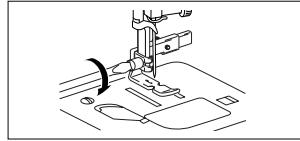
Attach the adjustable zipper/piping foot.
