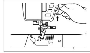
If it is difficult to feed thick fabrics under the presser foot, raise the presser foot to its highest position, and then raise the presser foot lever even further.
