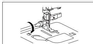
Attach the adjustable zipper/piping foot.
