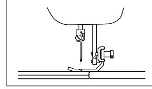
If the fabric will not feed at the beginning of sewing, place another piece of fabric with the same thickness under the back of the presser foot to level it.
